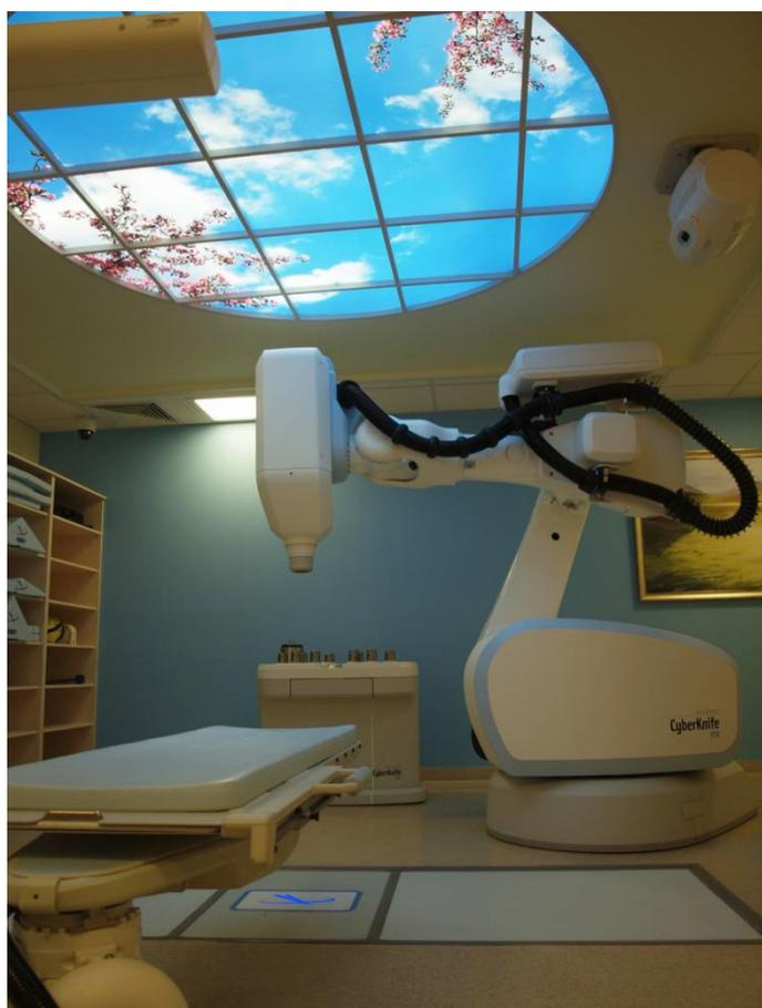
**Figure 1: Biomedical accelerator [A] for VMAT technique, equipped with a high-resolution multileaf collimator, [B] - CyberKnife equipped with wheel collimators. Both accelerators generates photon radiation (X-6 MV) and are equipped with the X-ray imaging. Despite the technical differences, these accelerators, are perfectly suited to the stereotactic radiosurgery implementation.**
