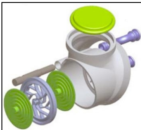
Figure 1: Exhalation valve system of GSR mask of SCOTT company [6]
