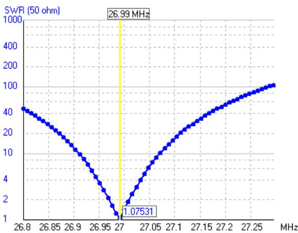
Fig. 6. The effect of the transformer over the VSWR (Voltage standing wave ratio)
