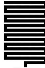
Fig. 7. Meandering antenna used in mobile devices like phones and tablets
