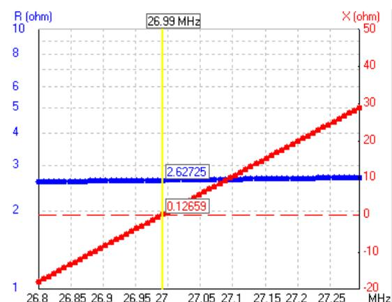
Fig. 3. Input impedance versus frequency
