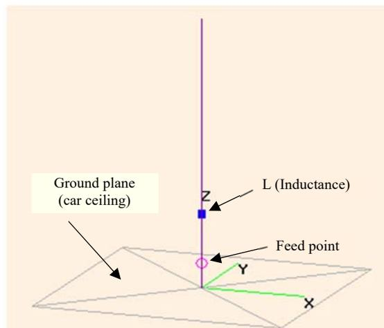
Fig. 2. High Q antenna in 4NEC2
