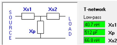
Fig. 5. The impedance transformer between load (antenna) and transmitter (source)
