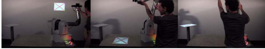
Fig. 5. Active Projection. The snapshots show how the user physically interacts with the robot for finding a suitable projection plane. The system aims to project a fixed size undistorted image following the geometric perspective of the projected surface
