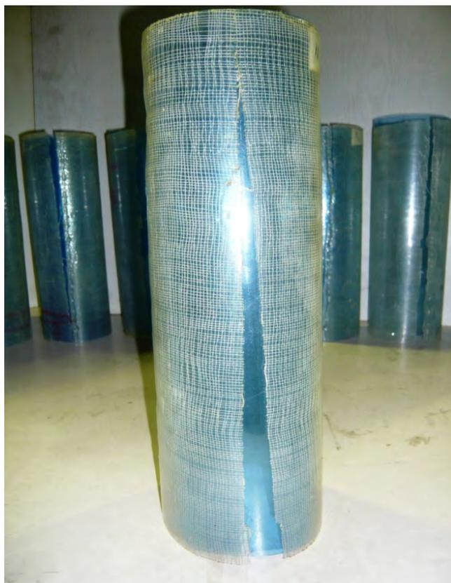
Figure 9. Tubular composite pipes after fracture (the blue transparent plastic sheet was put inside to be able to recognize the crack in the photo)
