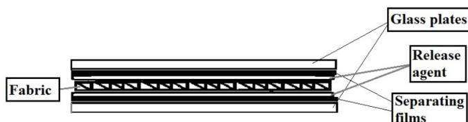
**Figure 2.** The set used for hand lay-up process of flat composite laminas
