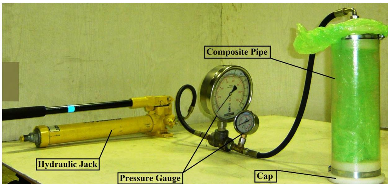
**Figure 6.** The set used for hydrostatic pressure test
