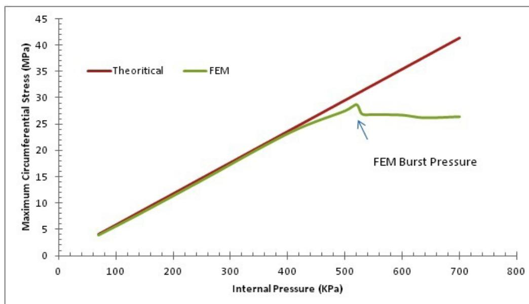
**Figure 10.** Maximum circumferential stress vs. internal pressure
