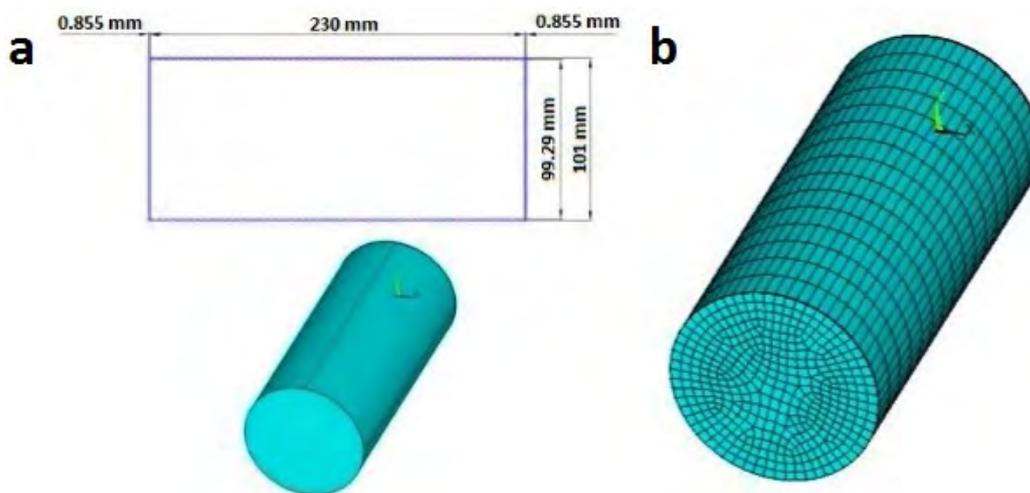
Figure 8. (a) Model geometry and (b) mesh schematic of close end shell
