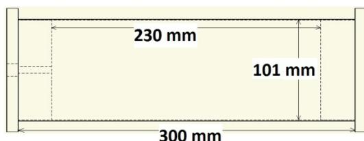
**Figure 5.** Dimensions of the produced composite pipes (including the caps)
