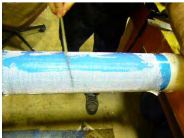
**Figure 3.** The mandrel used for producing composite pipe (while wetting the preform)
