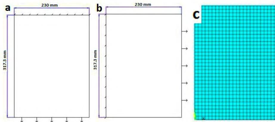
Figure 7. Model geometry and mesh schematic of the plate under tension, (a) warp dir., (b) weft dir., (c) mesh
