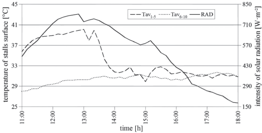
Figure 2. The course of the average temperature of surface of stalls 1–5 ( T_{av_{1-5}} ) and 6–10 ( T_{av_{6-10}} ) and intensity of solar radiation (RAD) over the study period
