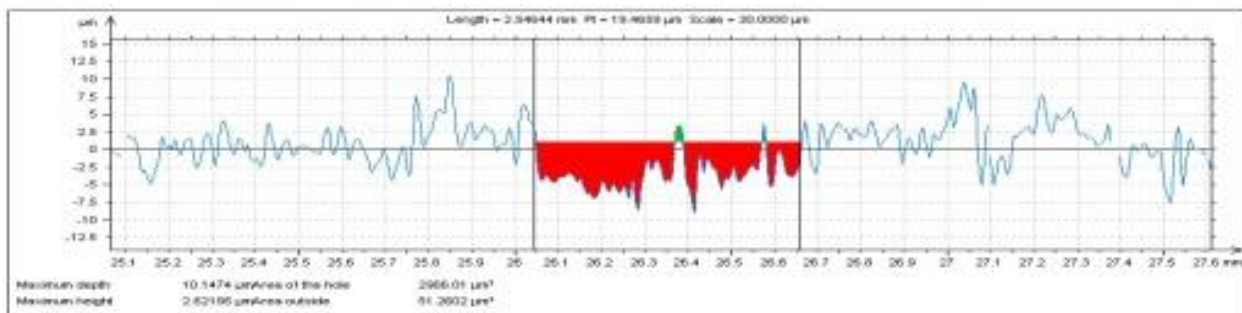
Fig. 4 Depth profile of coating 1350 wear trace
