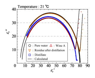
Fig.2 Measured and calculated Cole-Cole plots
