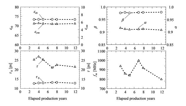
Fig.4 Dependence of Cole-Cole parameters on elapsed years
