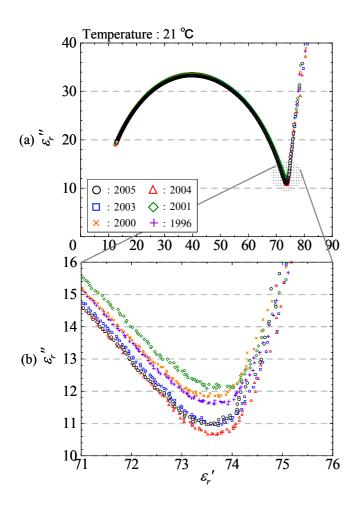
Fig.3 (a) Measured results of Cole-Cole plots for red wines of different production years and (b) enlargement of the Cole-Cole plots around minimum values
