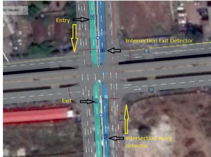
Figure 6. Signal and detector coordination in VISSIM
