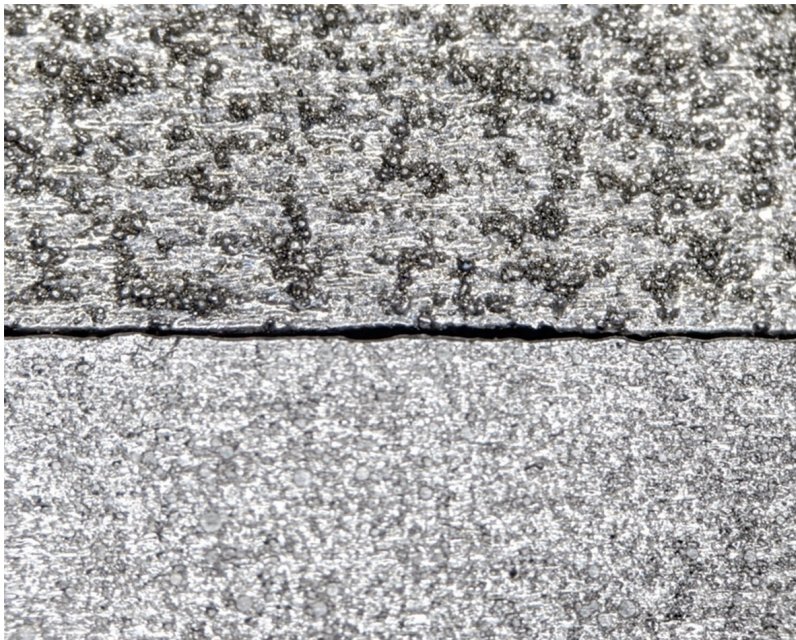
Fig. 17. Evidence of the balling effect was observed on sample No. 19 ( E_{dens} = 727 \text{ J/mm}^3 ). The top photo above shows a large number of balls on the side wall surface. For comparison, the effect is not noticeable on sample No. 4 ( E_{dens} = 105 \text{ J/mm}^3 ), where the printed surface is smooth.
