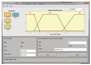
Fig. 7. LTs belonging to the input LVs of output voltage of the battery.
