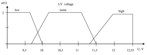
Fig. 1. Overlapping of LT of all range of LV "voltage".
