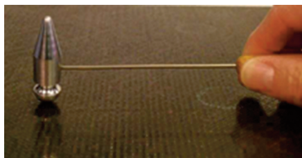
Fig. 5. Inspection of a composite structure by means of the tap lowering technique [15].
