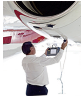
Fig. 3. Ultrasonic inspection of an aircraft during operation [11].
