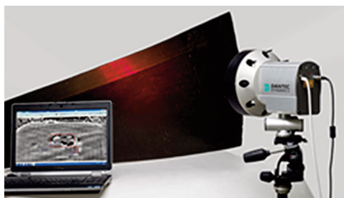
Fig. 6. Inspection of composite structure by means of the wide-graphic method [16].
