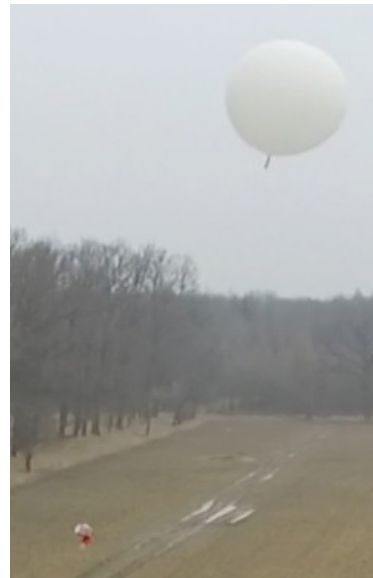
Fig. 2. a) The concept of connecting a gondola, parachute and balloon, which allows for the automatic activation of the parachute after cutting off the balloon [12], and b) the concept actually used in the mission - the balloon, regardless of the parachute, is permanently attached to the gondola.
