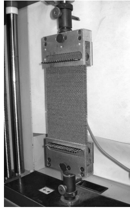
Fig. 10. Sample during test according to ASTM C363 [21]
