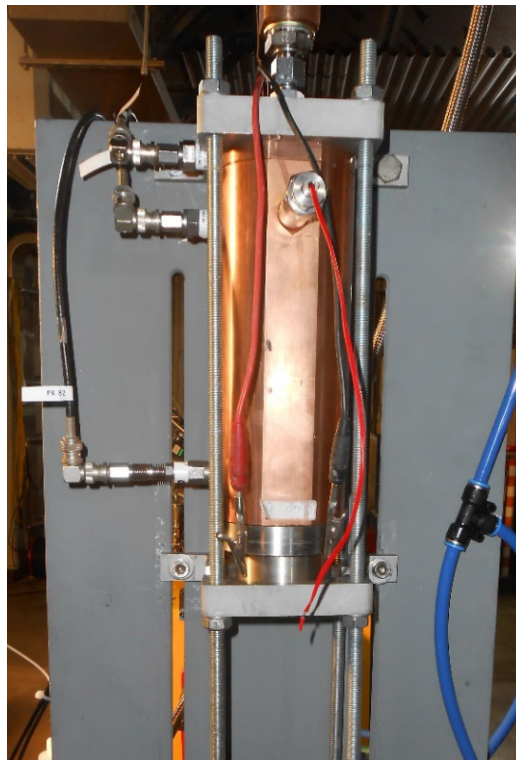
Figure 2 100N monopropellant test engine for the nitromethane engine firings
