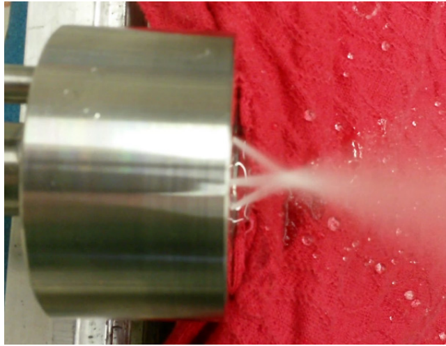
Figure 4: Fuel elements functional test with water and at ambient condition of the bi-propellant injector head
