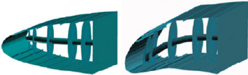
Fig. 2. The structural model of the wing in a standard position (left) and during deflection due to air pressure generated during flight (to the right) [4]
