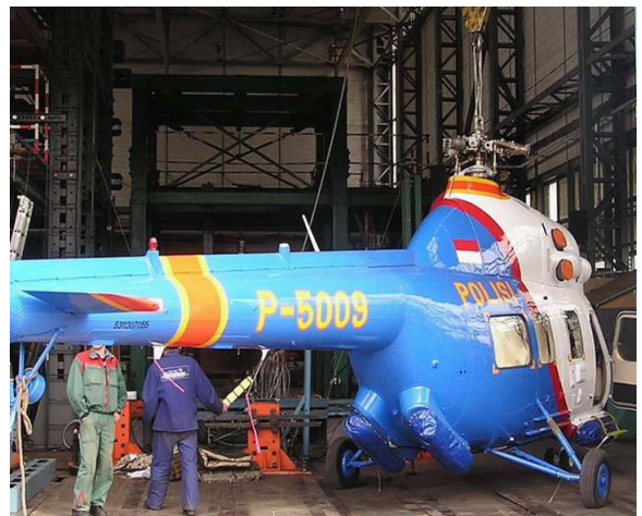
Fig. 7. Left - Mi-2 helicopter with floats designed by Władysław Burdan, Eng., during tests on Zemborzycki Reservoir, 1974. Right – Mi-2Plus for the Indonesian Police, with six emergency floats, 2006.
