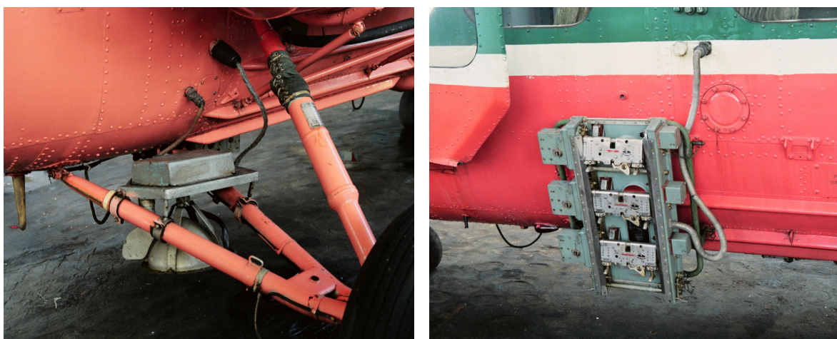
Fig. 4. Additional searchlights on the starboard side main landing gear strut, along with attachments for signaling bombs. Images: Miłosz Rusiecki
