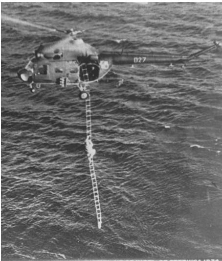
Fig. 10. Very good technical skills were required to climb aboard the helicopter using the rope ladder (left). It was impossible to use this method to lift an injured or an unconscious person. The image from the early stages of the helicopters' service life shows them sporting the original olive green liveries, the same as used on other military helicopters. Hydraulic, and then electric winches installed on the Mi-2RM made it possible to lower and hoist two people simultaneously - e.g. a rescuer and a victim (right). Images: WAF and Miłosz Rusiecki
