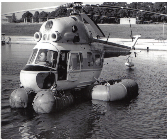
Fig. 7. Left - Mi-2 helicopter with floats designed by Władysław Burdan, Eng., during tests on Zemborzycki Reservoir, 1974. Right – Mi-2Plus for the Indonesian Police, with six emergency floats, 2006.
