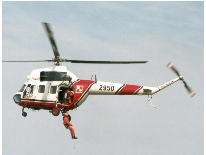
Fig. 10. Very good technical skills were required to climb aboard the helicopter using the rope ladder (left). It was impossible to use this method to lift an injured or an unconscious person. The image from the early stages of the helicopters' service life shows them sporting the original olive green liveries, the same as used on other military helicopters. Hydraulic, and then electric winches installed on the Mi-2RM made it possible to lower and hoist two people simultaneously - e.g. a rescuer and a victim (right). Images: WAF and Miłosz Rusiecki
