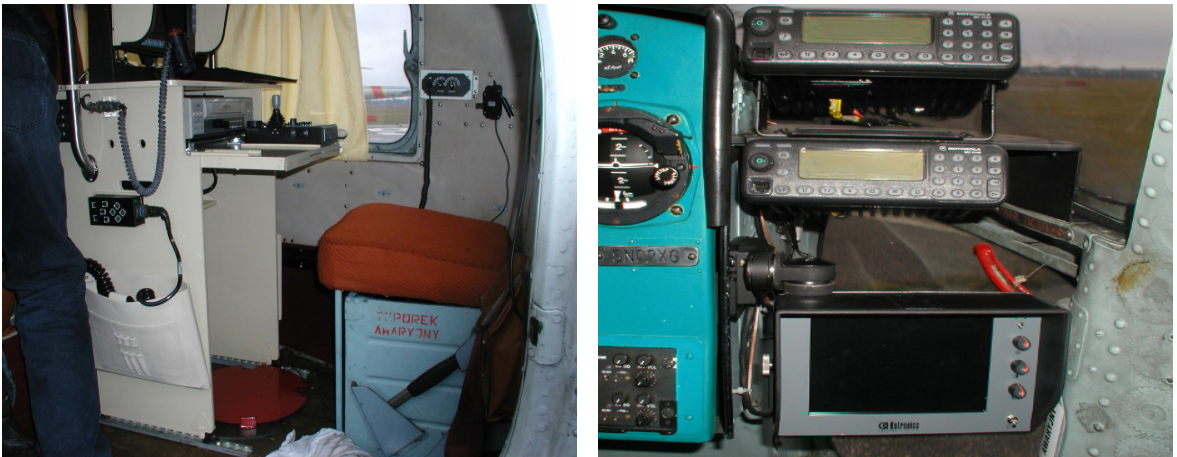
Fig. 8: left – station of the UltraForce 275 in-flight observation system operator; right – system's monitor used by the pilot, located under on-board radios. From the author's file.
