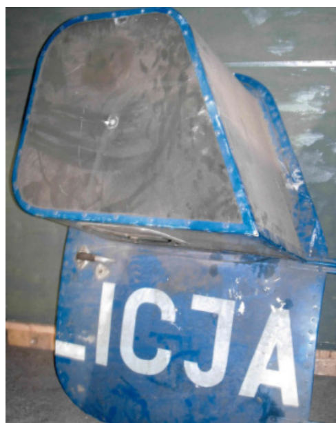
Fig. 3: Right-hand door of the Mi-2 helicopter enabling aerial images to be taken in a vertical position. Walenty Tiesłuk's file.
