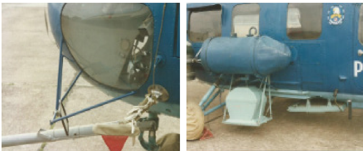
Fig. 5b: Special equipment: left – pilot's mirror; right – speaker and grenade launcher under the airframe. Marek Dominiak's file.
