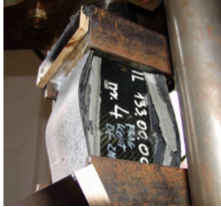
Fig. 9. FS after the static compression test [own elaboration, 2015]
