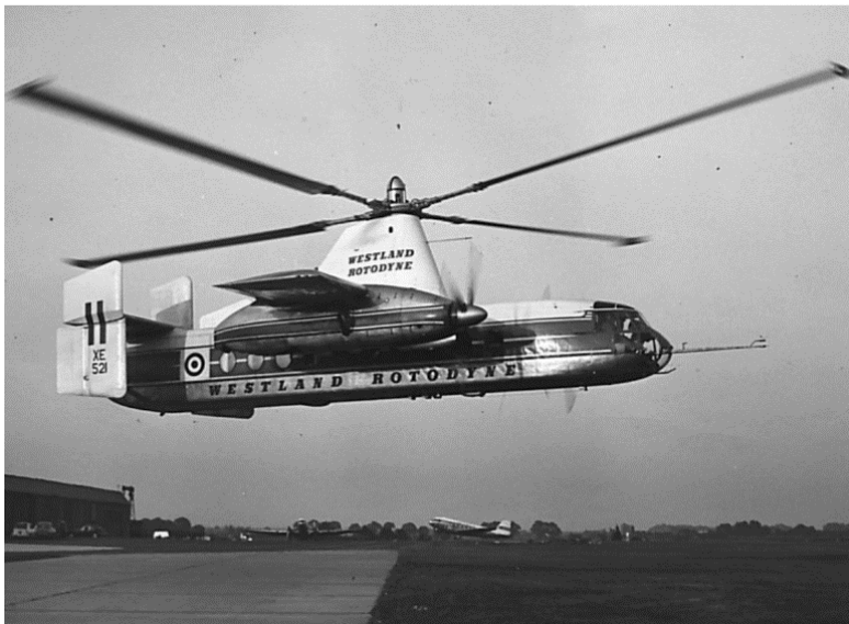
Fig. 9. Fairey Rotodyne as an example of gyrodyne [14].
