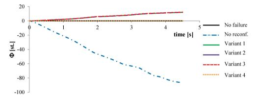
Fig. 9. Changes of the roll angle for the 2<sup>nd</sup> category of results [Żugaj, 2016]
