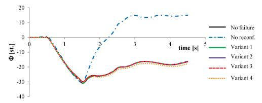
Fig.12. Changes of the roll angle for the 3<sup>rd</sup> category of results [Żugaj, 2016]
