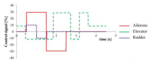
Fig. 4. Waveforms of the control input signals δ expressed as percentages of their maximum values [Żugaj, 2016]
