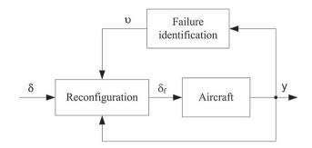
Fig. 3. The general diagram of the control system [Żugaj, 2016]
