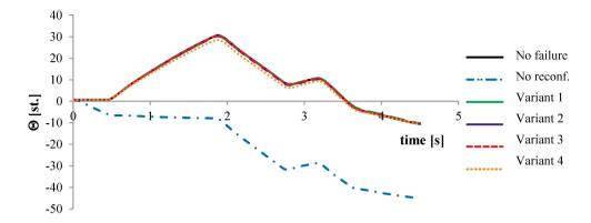
Fig. 5. Changes of the pitch angle for the 1st category of results [Żugaj, 2016]
