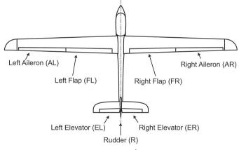
Fig. 2. Control System Configuration [Żugaj, 2014]
