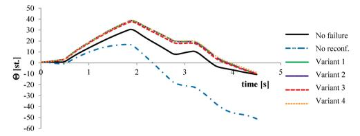
Fig. 8. Changes of the pitch angle for the 2<sup>nd</sup> category of results [Żugaj, 2016]
