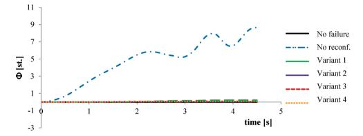
Fig. 6. Changes of the roll angle for the 1st category of results [Żugaj, 2016]
