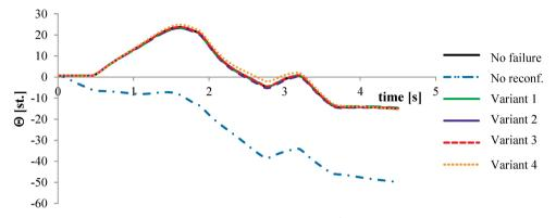
Fig. 11. Changes of the pitch angle for the 3rd category of results [Żugaj, 2016]
