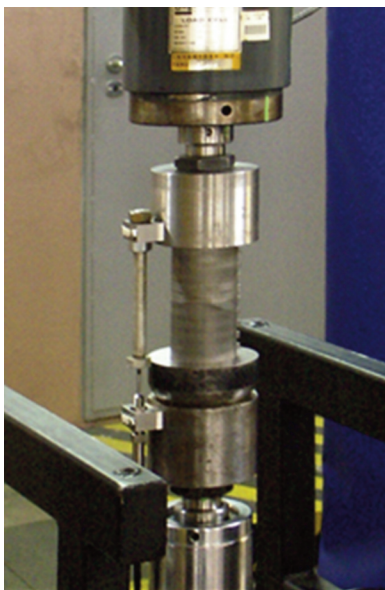
Fig. 2. Package of sheets during compression testing in the testing machine [Author, 2015]
