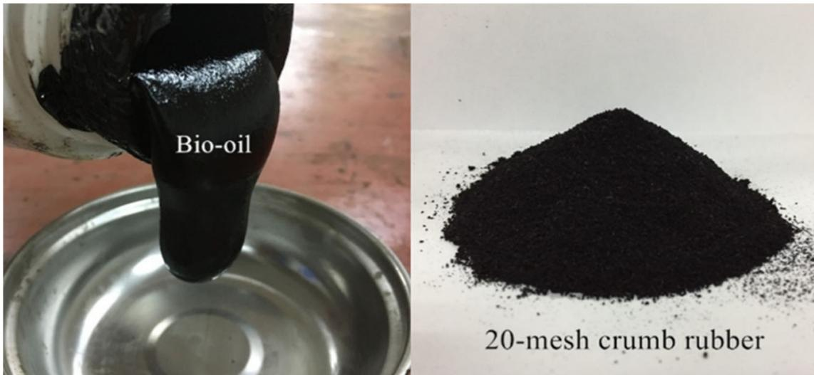
Figure 4: Used bio-oil and crumb rubber.
