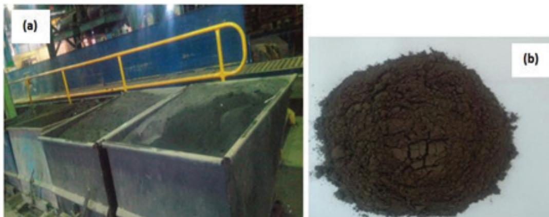
**Figure 1:** Foundry sand wastes used in this work: (a) rejected zone, (b) FSW as sand.
