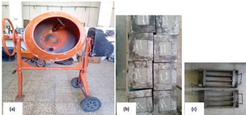
**Figure 8:** Mixer and molds used for self-compacting concrete: (a) concrete mixer, (b) cubic samples (150x150x150 mm<sup>3</sup>), (c) prismatic samples (70x70x280 mm<sup>3</sup>).
