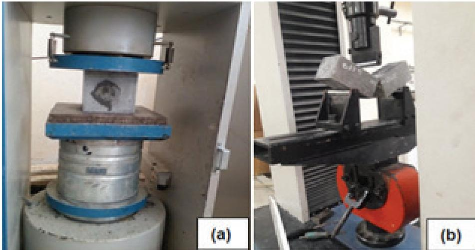
Figure 9: Mechanical tests: (a) compressive, (b) flexural strength.
