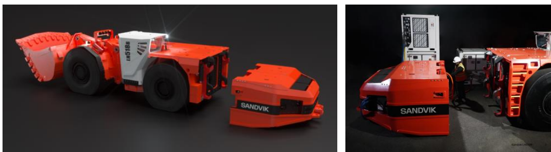
Fig. 3 LH518B loader with a quick battery replacement system
