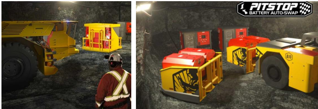
Fig. 2 Artisan quick battery replacement system - auto swap
