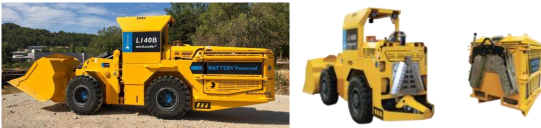
Fig. 9 Aramine L140B loader and QRS battery replacement system
