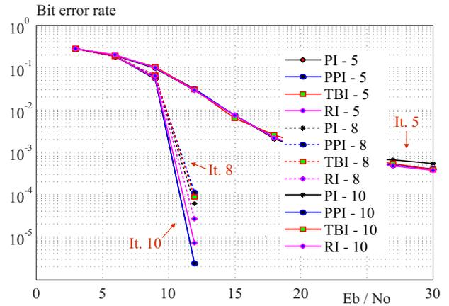
Fig. 5. BER performance for iteration count of 5, 8 and 10
