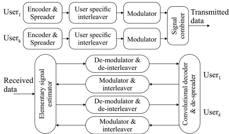
Fig. 1. IDMA transmitter and receiver system
