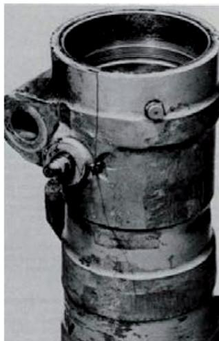
*Fig. 5. Crack resulting from undetected stress corrosion [19]*
