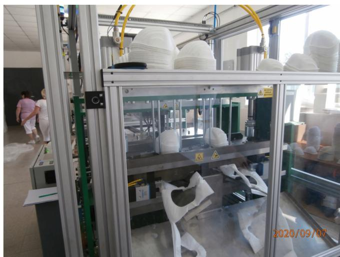
**Fig. 2.** Automated extrusion line for nanotextile respirators.
