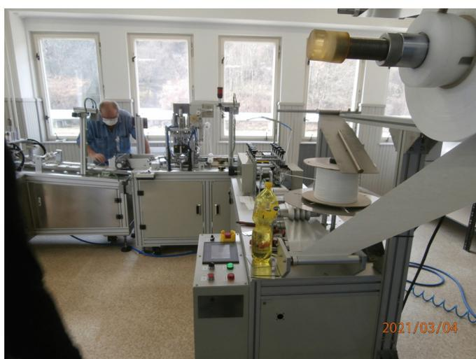
**Fig. 3.** Automated line for nanofiber masks Nanovia Mask 99,97 production.
