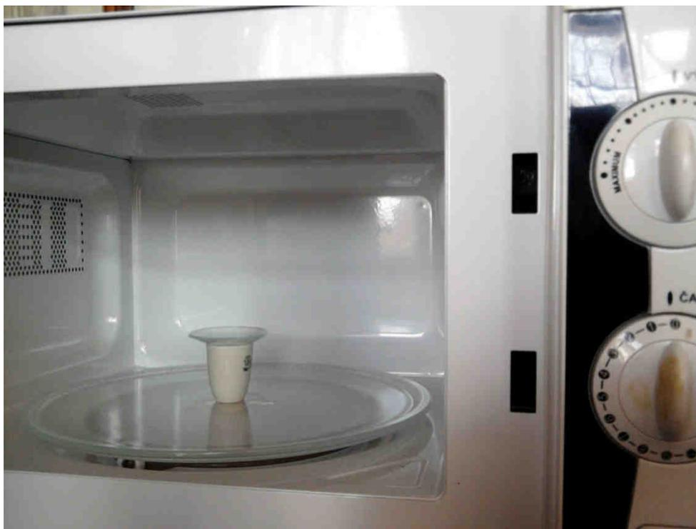
Fig. 2. Solvent-free synthesis of sulfanilic acid in microwave oven
