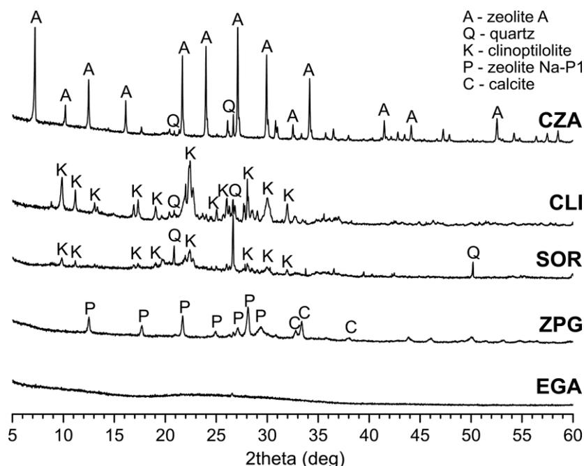
Fig. 2. X-ray diffraction patterns of materials used for sorption tests (A – zeolite A, Q – quartz, K – clinoptilolite, P – zeolite Na-P, C – calcite).
