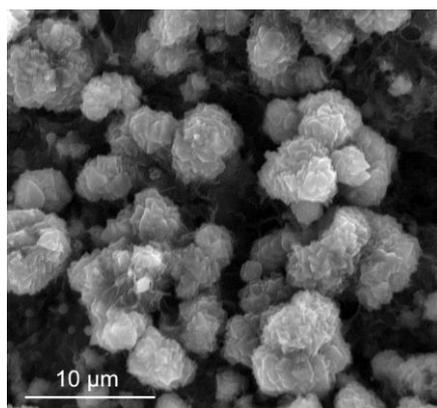
Fig. 1. Microstructure of ZPG observed in scanning electron microscope with crystallites of zeolite Na-P1.
