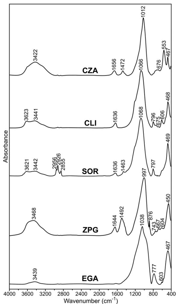
Fig. 3. FT-IR spectra of materials used for sorption tests.
