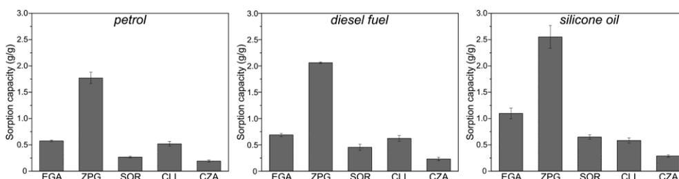
Fig. 4. Sorption capacities of materials used for the sorption of gasoline, diesel and silicone oil.
