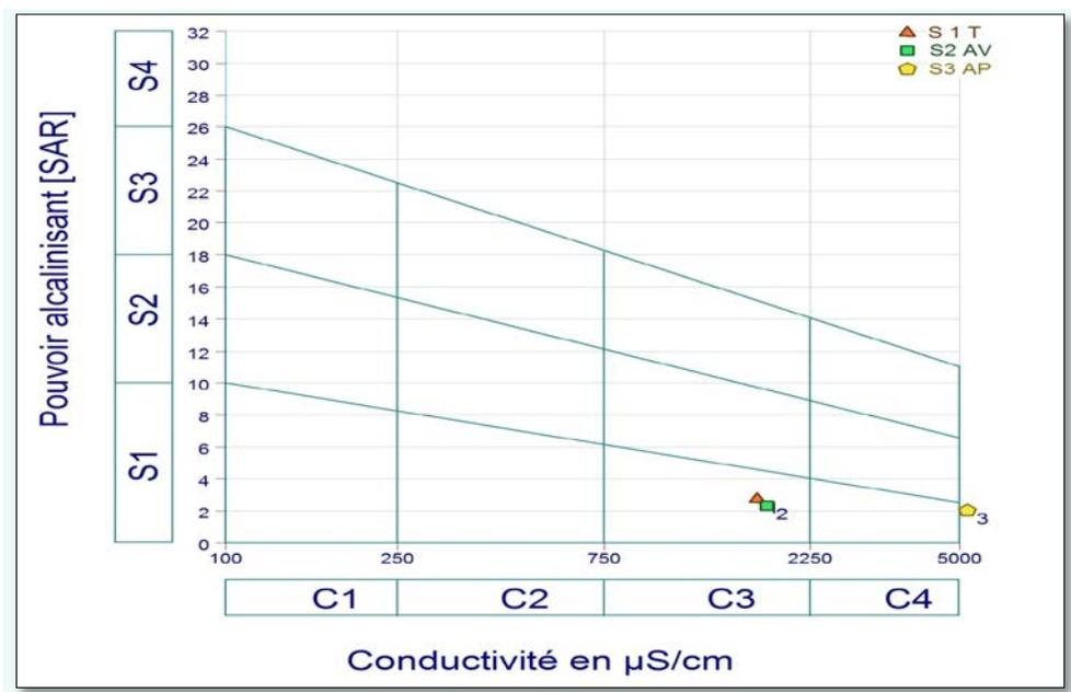
Figure 4: Diagram of Riverside for the classification of water of Meskiana River.
