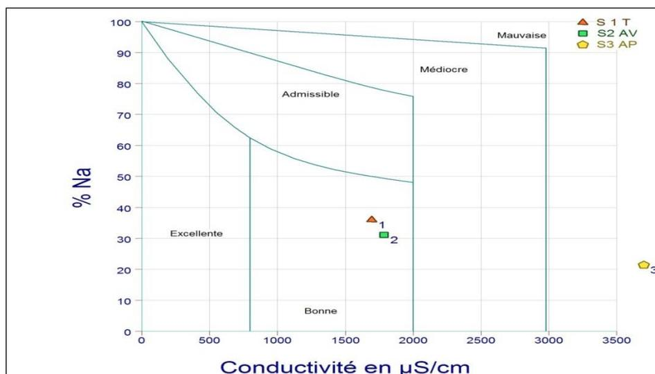
Figure 5: Diagram of Wilcox for the classification of water of Meskiana River.
