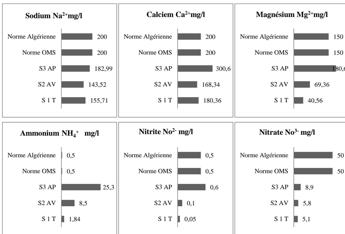
**Figure 3:** Results of the physicochemical analyses of the water of Meskiana Oued intended for irrigation.
